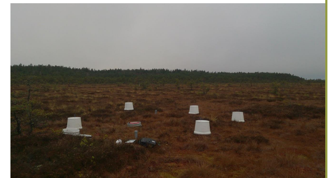
Sampling equipment – rings and chambers for collection of GHG.
