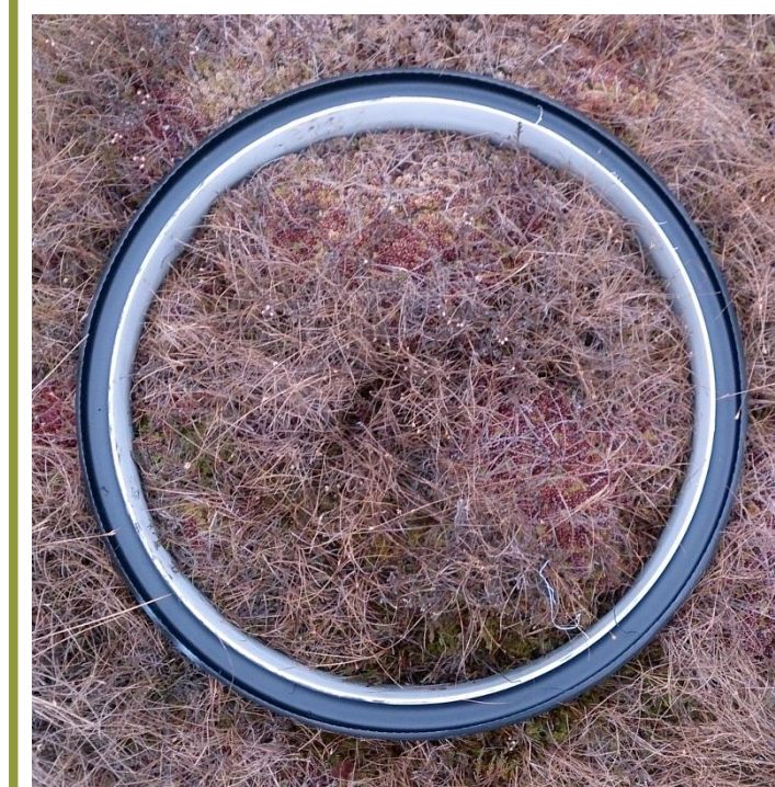
Sampling equipment – rings and chambers for collection of GHG.
